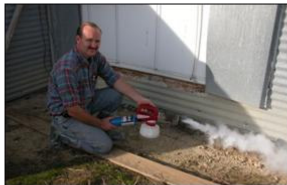
Photo 3: Generate smoke outside the house near the top of the foundation to see how much leaks into the house.
