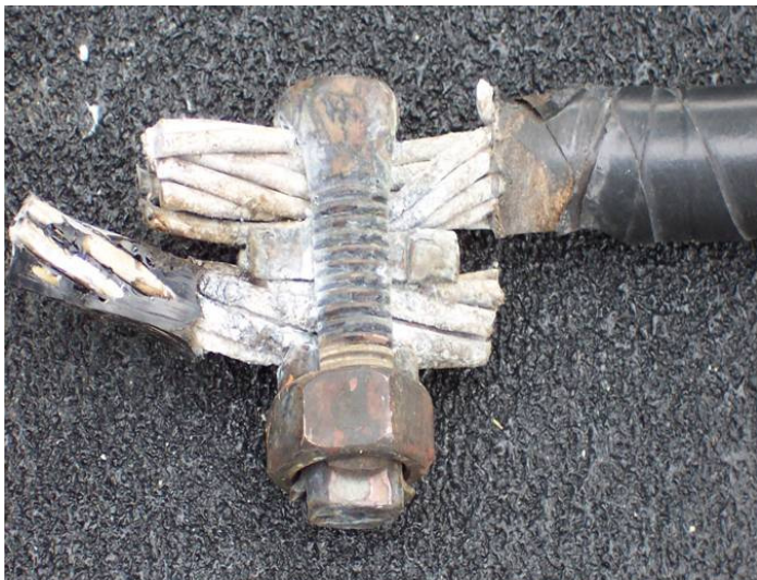
Photo 3: Wires incorrectly connected with a split bolt connector.
