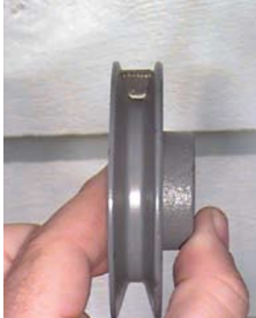
Figure 1. A worn fan belt riding low in the pulley reduces the effective pulley size. This belt should be replaced.
