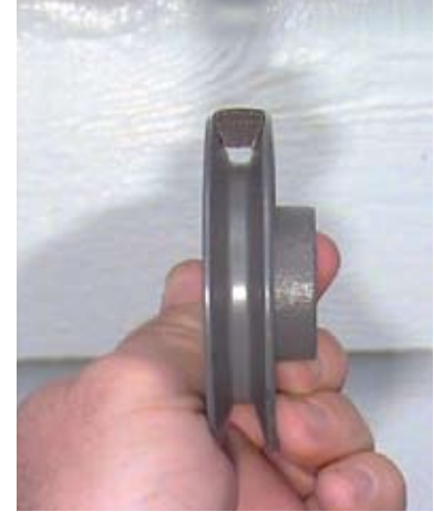
Figure 2. A new fan belt rides high in the pulley so that the top of the belt rides just above the top of the pulley.
