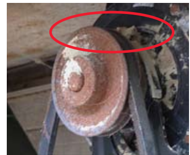
Figure 4. A front view of a worn belt riding low in the pulley
